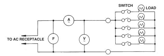
Use a circuit above for measuring AC output. A hot plate or lamp with a power factor of 1.0 may be used as a load. Adjust the load and rpm, and check that the voltage range is as specified in the following table at the rated amperage and rated rpm.
