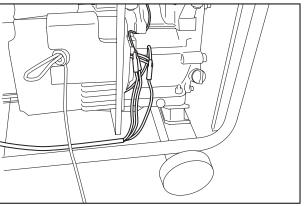
(4) Install the regulator to the battery box.M6 x 8mm Flange bolt : 1 pce.
