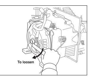
(2) Using a special tool, Rotor Puller, remove the rear cover together with rotor and stator.
