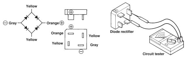
The circuit inside the diode rectifiers is as shown in the chart above.
