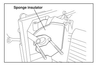
(2) Install the Carburetor to the intake flange.
