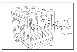
(3) Loosen the five bolts and remove the cover bracket from the inverter unit.
