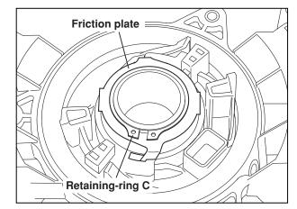
(3)Installation of friction plate and retaining ring C. Install by putting the Tab of friction plate into the hole of the ratchet.
