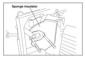
(2) Loosen the two M6 nuts and one M6 bolt, and remove the air cleaner body.
