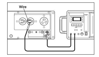
Any part where the insulation resistance is less than  $1M\Omega$  has faulty insulation, and may cause electric leakage and electric shock.
